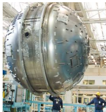
Figure 6. A Lightweight, Disposable “Pre-Depot” Tank, Derived from Centaur LO 2 Tank, with 26 mT LO 2 Capacity. Credit ULA
