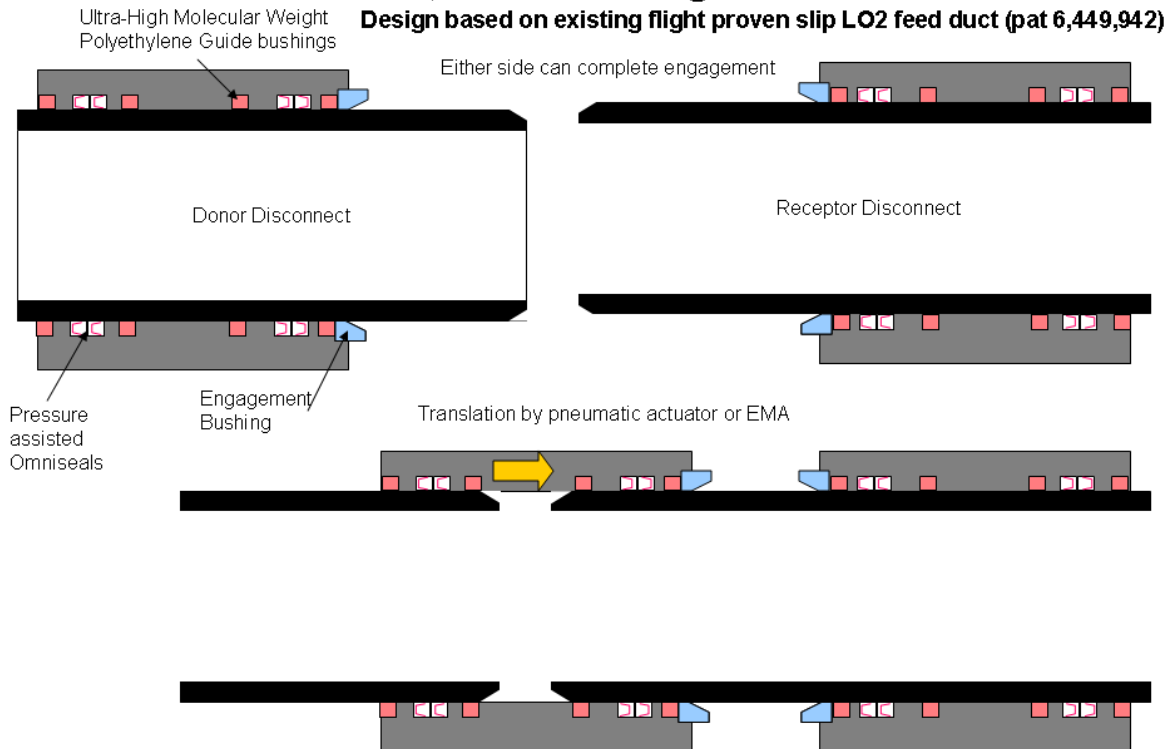
Figure 5. Illustration of a Slip-Joint Duct Connector for Cryogenic Propellant Transfer. Credit ULA
